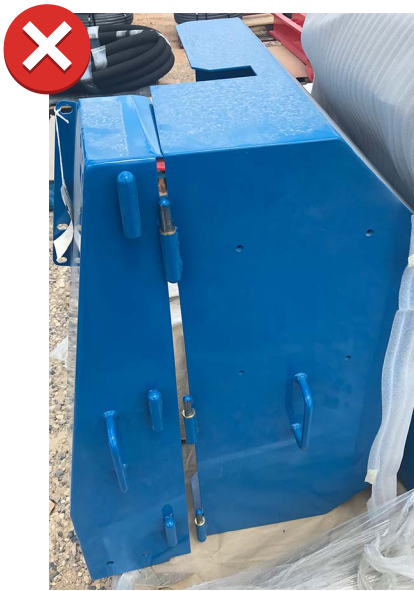
Hinges welded incorrectly (Pin must not be facing up on door)
