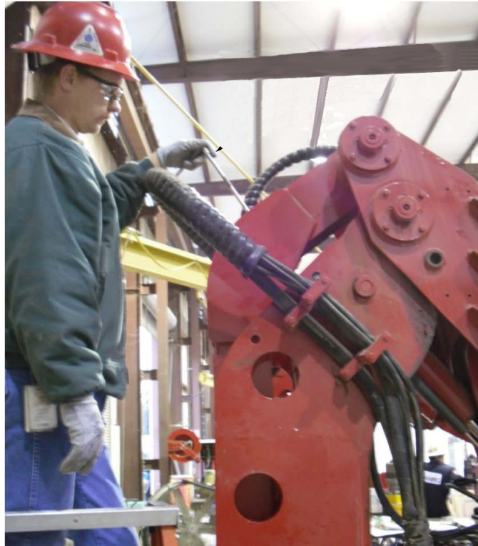
Figure 9: Keep the Ratchet Clear of Hoses and Cables
