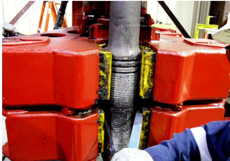
Figure 3: Prying the Lower Clamp Cylinders off the Pipe
