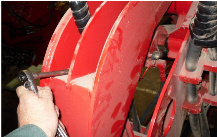
Figure 8: Slowly Turn the Counterbalance Valve Clockwise
