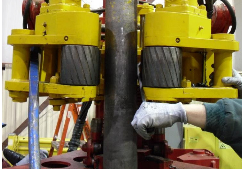
Figure 4: Prying the Spinner Clamps Away from the Pipe
