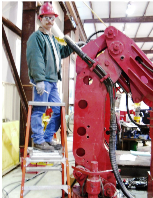
Figure 6: Proper Ladder Placement
